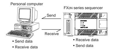
• Use the communication cable suited to the connector pin configuration of the personal computer.
