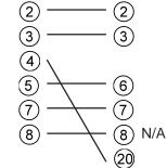
NOTE: The FX0N-232ADP does not monitor the CD pin (pin 8).
