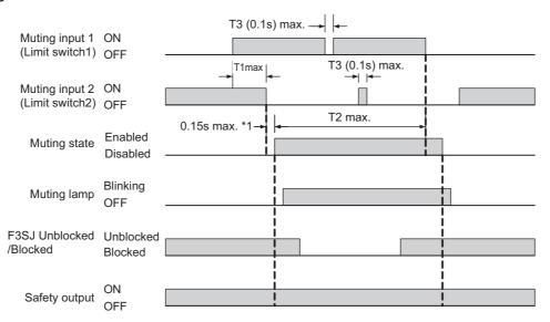
\*1 The value is applied to a single sensor. Values for connected sensors are:
