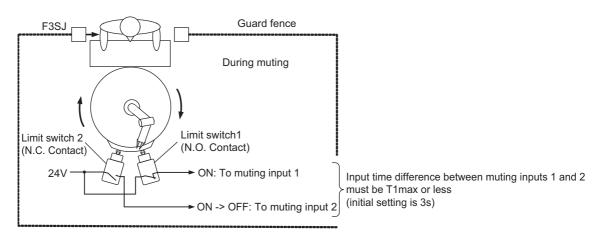
When the muting input 1 turns from OFF to ON and when the muting input 2 is turned from ON to OFF within T1max [s] before or after the muting input 1's turning ON, safety function of F3SJ is disabled. (Safety output is kept ON even if F3SJ is blocked)
