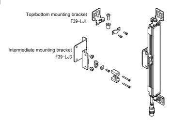
The adjustment angle of F39-LJ3 is from -10deg to +10deg.
