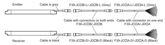
■ Cable with Connectors on Both Ends: Cable for Connection with G9SA-300-SC (F39-JC□C, sold separately)
