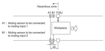
A workpiece finished passing the muting sensor A1 and the sensor starts turning OFF. For standard muting system, muting is released here. For exit only muting, F3SJ's safety function is disabled for a exit only muting delay time: T5.
