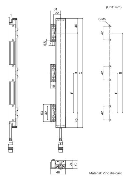
Side mounting (when using intermediate brackets for side mounting)
