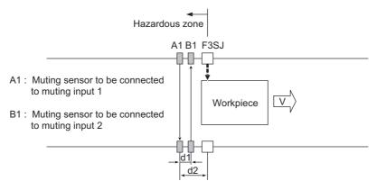
A workpiece finished passing the muting sensor B1 and the sensor is turned OFF. F3SJ disables its safety function if it is within a exit only muting delay time.
