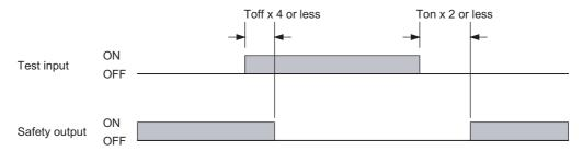
Ton: Response time of safety output's OFF to ON, Toff: Response time of safety output's ON to OFF
