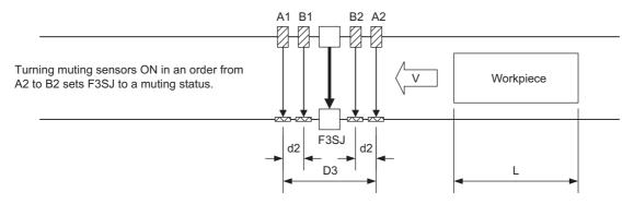
This arrangement example uses regressive reflection type E3Z-RDD series as a muting sensor. Arrangement must take mutual interference into account.
