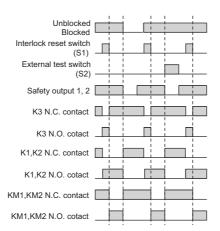
Note 1) F3SJ's external device monitoring and auxiliary output cannot be used. Note 2) S2 performs normal operation when opened and external test when short-circuited. Note 3) Do not connect any cable to terminals C1, D1, D2, E1, and E2
