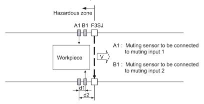
When muting sensors A1 and B1 are turned ON in this order, and the muting function is enabled. In this state, the safety function of F3SJ is disabled.
