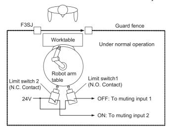
The limit switch 1 of N.O contact is open and the muting input 1 is OFF, and the limit switch 2 of N.C contact is short-circuited and the muting input 2 is ON, and safety function of F3SJ is being enabled.
