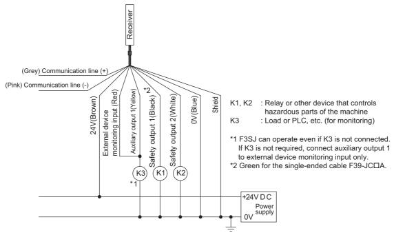
■ Ref.: Minimum Wiring Required to Check the Operation of the F3SJ When Using the Muting Function
