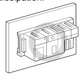
(b) Do not use the programmable controller in the following positions:
